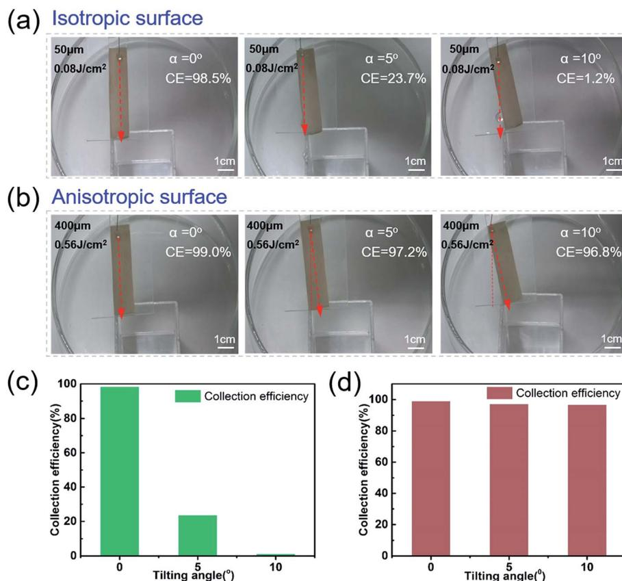
Fig. 5 Comparison of the liquid collection efficiency on isotropic and anisotropic surfaces under different rotation angles. (a) and (b) Water collection with rotation angles of 0, 5,  $10^\circ$  on isotropic surface and anisotropic surface. (c) and (d) Water collection efficiency histogram of the isotropic surface and anisotropic surface.
