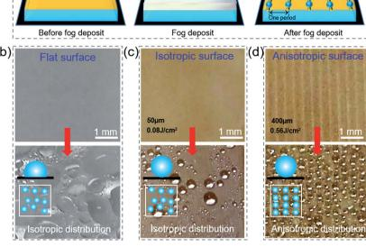
Fig. 6 Directional and size-constrained fog deposition. (a) Schematic of the fog deposition process. (b)-(d) Images of flat, isotropic and anisotropic surfaces before and after fog deposition. The inset schematic images indicate the contact and distribute mode of each surface.
