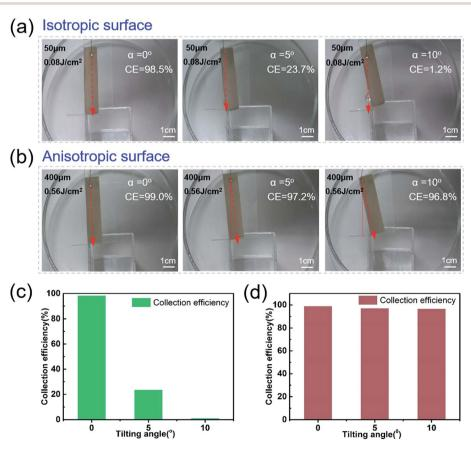
Fig. 5 Comparison of the liquid collection efficiency on isotropic and anisotropic surfaces under different rotation angles. (a) and (b) Water collection with rotation angles of 0, 5, 10° on isotropic surface and anisotropic surface. (c) and (d) Water collection efficiency histogram of the isotropic surface and anisotropic surface.
