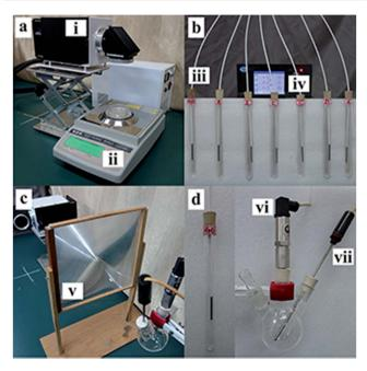
Fig. 2 The accessible experimental setups for testing the photo-thermal conversion including (a) mass loss rate testing, (b) heating rate testing, (c) pressure rise rate testing and (d) details of pressure testing. The main instruments include (i) xenon lamp, (ii) electronic balance, (iii) temperature-measuring thermocouple, (iv) temperature recorder, (v) Fresnel lens, (vi) pressure transducer and (vii) rod-like thermocouple.
