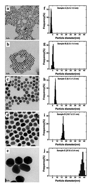
Fig. 3 TEM images and size distributions of gold nanoparticles: (a) and (f) for sample A (3.4  $\pm$  1.3 nm), (b) and (g) for sample B (5.3  $\pm$  1.4 nm), (c) and (h) for sample C (8.1  $\pm$  1.3 nm), (d) and (i) for sample D (16.7  $\pm$  2.1 nm) and (e) and (j) for sample e (37.8  $\pm$  3.4 nm).
