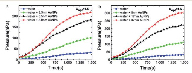
Fig. 10 The pressure changes over time of Au nanoparticles from G1 (a) and G2 (b) under 1.5 kW m<sup>-2</sup> solar illumination.
