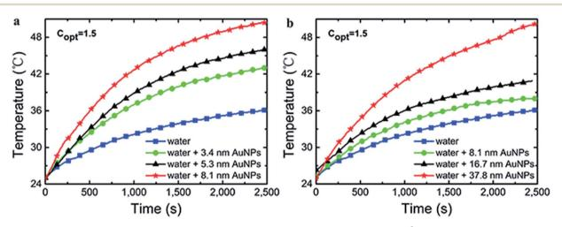
The temperature changes with time for Au NPs fluids from G1 (a) and G2 (b) under 1.5 kW m<sup>-2</sup> illumination.
