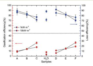
Fig. 6 The vaporazation efficiency and loss efficiency of pure water and Au NPs dispersions with different diameters (sample A to F) under solar illumination with 1 and 10 kW  $\rm m^{-2}$ , respectively.
