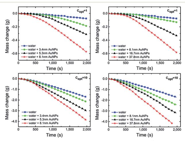
Fig. 5 The mass loss (evaporated water) of Au NPs dispersions with different diameters under 1 and 10 kW m<sup>-2</sup> xenon lamp's illumination compared with pure water. Au NPs from G1 (a) and G2 (b) were irradiated under  $1 \text{ kW m}^{-2}$  illumination. Similarly, Au NPs from G1 (c) and G2 (d) were irradiated under 10 kW m<sup>-2</sup> illumination.
