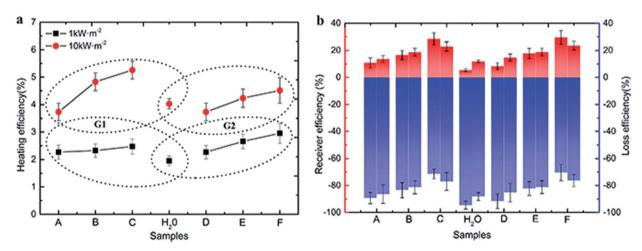
Fig. 8 Three kinds of efficiencies for photothermal conversion. (a) Heating efficiency of Au nanoparticles from G1 and G2 under 1 and 10 kW m $^{-2}$  solar illumination. (b) Receiver efficiency and loss efficiency of Au nanoparticles from G1 and G2 under 1 and 10 kW m $^{-2}$  illumination.
