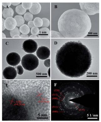
Fig. 2 (A and B) SEM images, (C and D) TEM images, (E) HRTEM image and (F) the corresponding SAED pattern of the ZnCo<sub>2</sub>O<sub>4</sub> microspheres.
