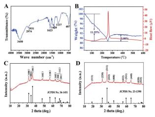
Fig. 1 (A) The FT-IR spectrum of the ZnCo-precursor. (B) The TG and DTA curves obtained for the ZnCo-precursor. (C) The XRD pattern of the ZnCo-precursor. (D) The XRD pattern of ZnCo<sub>2</sub>O<sub>4</sub>.
