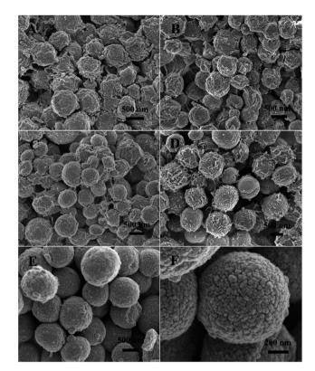
Fig. 3 SEM images of the ZnCo-precursor prepared under different grown conditions: (A) 2 h, (B) 4 h, (C) 6 h, (D) 8 h, and (E and F) 10 h.
