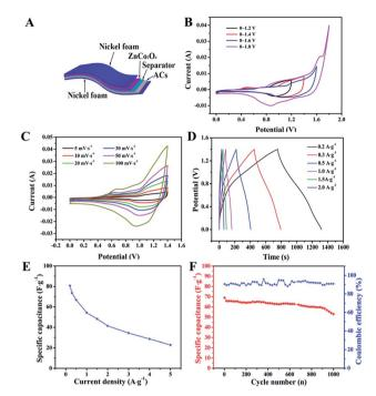
Fig. 6 (A) A schematic of the  $\rm ZnCo_2O_4//AC$  quasi-solid-state asymmetric supercapacitor. (B) CV curves obtained at different potential windows. (C) The CV curves obtained at various scan rates. (D) The GCD attributed to some irreversible reactions occurring in the potential curves under different current densities. (E) The specific capacitance of the device as a function of current density. (F) The cycling performance and the corresponding Coulomb efficiency at 0.5 A g $^{-1}$ .
