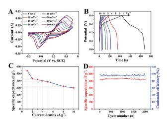
Fig. 5 The electrochemical test results of the  $ZnCo_2O_4$  microsphere electrode. (A) The CV curves at various scan rates. (B) The GCD curves at various current density. (C) The capacitance as a function of current density. (D) The cycling performance and Coulomb efficiency at 2 A g $^{-1}$ .
