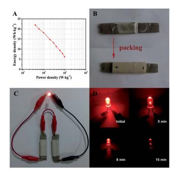
Fig. 7 (A) Ragone plots of the  $ZnCo_2O_4//AC$  quasi-solid-state asymmetric supercapacitor. (B) Digital photographs of the  $ZnCo_2O_4//AC$  quasi-solid-state asymmetric supercapacitor before and after packing. (C) Optical images of a red LED powered by two solid-state asymmetric supercapacitors connected in a series. (D) The evaluation of the lightened red LED at different stages after corresponding to (C).
