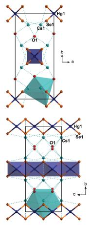
Fig. 2 Fragments of the crystal structure of 2, viewed along (001) (top) and (100) (bottom). The coordination polyhedra around the Hg atoms of the central strand and around one Cs atom are shown. All atoms are drawn with displacement ellipsoids at the 50% probability level.
