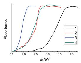
Fig. 5 UV-Visible spectra of compounds 1–4. The following  $E_{onset}$ values were determined by means of the tangent method: 2.9 eV (1); 2.4 eV (2); 1.7 eV (3); 2.1 eV (4). Note that the onset of absorption for compound 2 is intrinsically red-shifted due to the beginning of decomposition of the very sensitive compound during sample preparation; for this, only the sharply ascending part of the curve was used to determine the optical gap.
