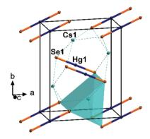
Fig. 1 Fragment of the crystal structure of 1, viewed approximately along  $\langle 00\overline{1}\rangle$ . The coordination polyhedron of one Cs atom is shown. All atoms are drawn with displacement ellipsoids at the 50% probability level.
