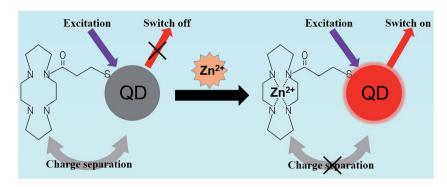
**Fig. 6** Schematic principle of zinc ion nanosensors. Conjugation of QDs and azamacrocycles causes charge separation and quenching of QDs. The complexation of Zn(II) with the ligand changes the energy level on the ligand, which prevents the charge separation and leads to the fluorescence recovery of QDs. Reproduced from ref. 106 with permission. Copyright © 2008, American Chemical Society.
