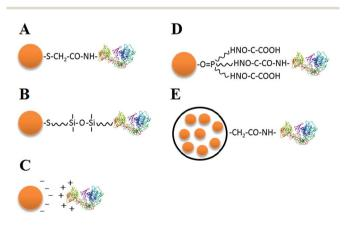
Fig. 2 Common bioconjugation strategies of QDs, including connection between carboxyl and amino  $(-COOH \text{ and } -NH_2)$  functional groups of bifunctional molecules (A), functional group linkage of typical silane compounds (B), electrostatic interaction (C), linkage between hydrophilic and hydrophobic groups (D), and the use of functionalized microbeads as conjugation media (E). A, B, and D belong to the category of covalent linkage strategies.
