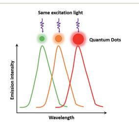
**Fig. 1** Emission spectra of QDs with different sizes under the same excitation light. Each spectrum was normalized to the peak emission. There is a red-shift of QD emission wavelength as the size of the QD increases. The emission spectra of QDs are symmetrical without red tails.
