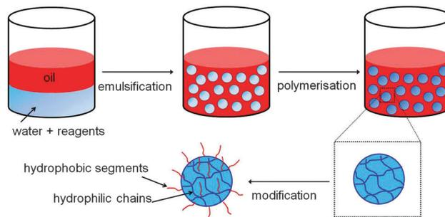
Fig. 1 Schematic illustration of the most common approach to amphiphilic microgel production *via* emulsion templating and post-modification of the microgel. The hydrophobic and hydrophilic moieties are coloured in red and blue, respectively.
