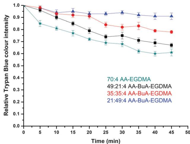
Fig. 11 Hydrophilic dye release in neutral pH solution ( $\sim$ pH 7). The plots show the relative Trypan Blue colour intensity versus time for each variation of the AA–BuA–EGDMA microgels. Green stars, black squares, red circles and blue triangles represent microgels with 70 : 0 : 4, 49 : 21 : 4, 35 : 35 : 4 and 21 : 49 : 4 AA : BuA : EGDMA molar ratios, respectively.
