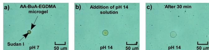
Fig. 8 (a) AA<sub>49</sub>-co-BuA<sub>21</sub>-co-EGDMA<sub>4</sub> microgel with hydrophobic Sudan I dye encapsulated inside at pH 7. (b) The same microgel immediately after addition of pH 14 solution, and (c) 30 min after addition of pH 14 solution.
