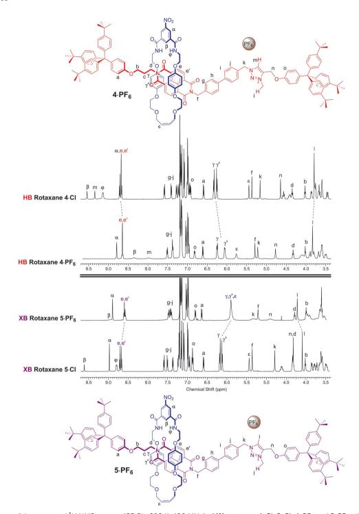
Fig. 3 Comparison of the truncated  $^1H$  NMR spectra (CDCl $_3$ , 298 K, 400 MHz) of [2] rotaxanes  $4 \cdot Cl$ ,  $5 \cdot Cl$ ,  $4 \cdot PF_6$  and  $5 \cdot PF_6$  with their predicted co-conformations in the presence of  $PF_6$ .
