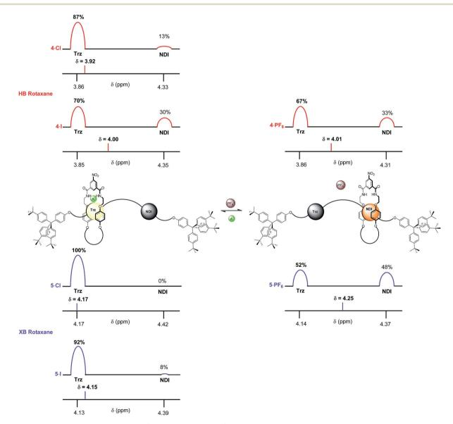
Fig. 8 The estimated percentage occupancies (based upon  $H_1$  protons) of the HB and XB rotaxanes  $4 \cdot A$  and  $5 \cdot A$  as chloride, iodide and  $PF_6$  salts as determined by  $^{1}H$  NMR spectroscopy in 4 : 1 CDCl<sub>3</sub> : CD<sub>3</sub>OD solution.  $A^{-} = Cl^{-}$  or  $I^{-}$  and Trz = triazolium.
