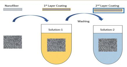
Fig. 9 Layer-by-layer treatment for functionalization of electrospun fibers.
