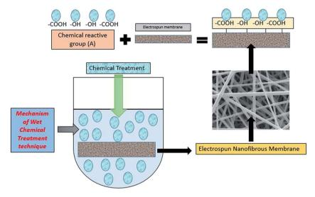
Fig. 10 Wet chemical treatment for functionalization of electrospun fibers
