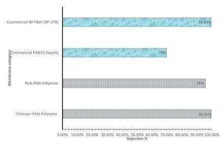
Fig. 13 Comparative study of rejection% of various membranes. [Note: mid layer of 3 tier membrane system is PAN (electrospun membrane), feed solution: mixture of vegetable oil (1350 ppm), surfactant (150 ppm, Dow Corning 193 fluid) and deionized water. Plotted the figure by using the data. [18]
