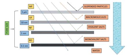
Fig. 4 Size of different particulates rejected by various membrane processes.<sup>32</sup>
