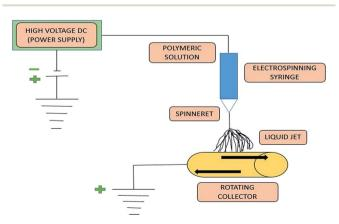
Fig. 1 Schematic block diagram of electrospinning technique.
