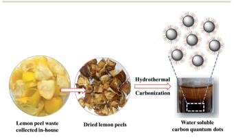
**Scheme 1** Schematic illustration for the synthetic procedure of wsCQDs by hydrothermal treatment of lemon peel waste precursor.
