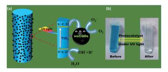
Fig. 8 (a) Schematic illustration for the photocatalytic degradation of MB on  $TiO_2$ –wsCQDs composite under UV light irradiation and (b) digital images of MB before and after degradation.
