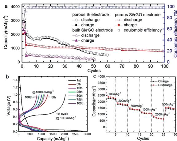
Fig. 15 (a) Cycle performance at a constant current rate of 1000 mA g<sup>-1</sup> after initial activation processes at 100 mA g<sup>-1</sup> for two cycles; (b) galvanostatic discharge–charge profiles; and (c) rate performance of Si/graphene composite electrode.<sup>171</sup> Reprinted (adapted) with permission from ref. 171. Copyright (2015) American Chemical Society.
