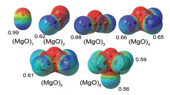
Fig. 2 Molecular electrostatic potential (MEP) of the six  $(MgO)_n$  molecules  $(n=1\ \text{to}\ 6)$  studied. The MEP is shown on the 0.0004 electrons per bohr<sup>3</sup> density contour with a MEP scale ranging from -0.78 volts (red) to 0.78 volts (blue). The numbers appearing beside the terminal Mg atoms are their DDEC6 NACs.
