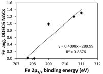
Fig. 4 Left: Correlation between Fe oxidation state and average Fe DDEC6 NAC for Fe, Fe<sub>2</sub>SiO<sub>4</sub>, Fe<sub>2</sub>O<sub>3</sub>, Fe<sub>3</sub>O<sub>4</sub>, and Fe<sub>3</sub>Si solids. Right: Correlation between 2p<sub>3/2</sub> core electron binding energy (as measured using XPS) and average Fe DDEC6 NAC for these materials.
