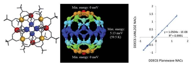
Fig. 9 Left: Atomic structure of  $Mn_{12}$ -acetate single molecule magnet. Mn type 1 (blue), Mn type 2 (red), Mn type 3 (yellow). In the minimum energy conformations, the Mn ASM vectors are perpendicular to the plane of the page. Middle: Computed spin-orbit coupling potential energy surface. Right: Comparison of DDEC6 NACs computed with LANL2DZ and planewave basis sets.
