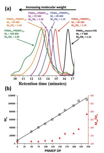
Fig. 2 (a) 3:1 Chloroform/methanol GPC curves obtained for PSMA<sub>14</sub>–PNMEP<sub>x</sub> diblock copolymer nanoparticles prepared at 10% w/w solids *via* RAFT dispersion polymerisation of NMEP at 90 °C. (b) Relationship between target PNMEP DP and GPC  $M_n$  (black squares) and  $M_w/M_n$  (red triangles) for the same series of PSMA<sub>14</sub>–PNMEP<sub>x</sub> diblock copolymer nanoparticles prepared at 10% w/w solids.
