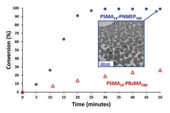
Fig. 1 Kinetics of the polymerisation of NMEP and BzMA at 90 °C when targeting PSMA<sub>14</sub>-PNMEP<sub>100</sub> (blue circles) and PSMA<sub>14</sub>-PBzMA<sub>100</sub> (red triangles) at 20% w/w solids. Insert: transmission electron microscopy image obtained after 50 min for PSMA<sub>14</sub>-PNMEP<sub>100</sub> showing the formation of near-monodisperse spherical nanoparticles with a mean diameter of 27 nm.
