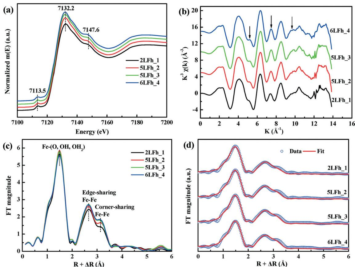
**Fig. 3** Fe K-edge XANES (a); the  $k^3$ -weighted EXAFS spectra, where the arrows indicate the main oscillations affected by the crystallite size (b); the Fourier transforms (magnitude) of the  $k^3$ -weighted EXAFS spectra (c); the radial distribution functions (symbols) and their fits using the Michel model (red curves) (d).
