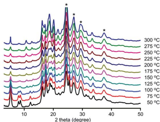
Fig. 2 Variable-temperature PXRD patterns for **DPT-MIDA**. The asterisks (\*) denotes the background signal from a polyether ether ketone layer that protects the detector. The temperature was recorded in 25 °C increments.
