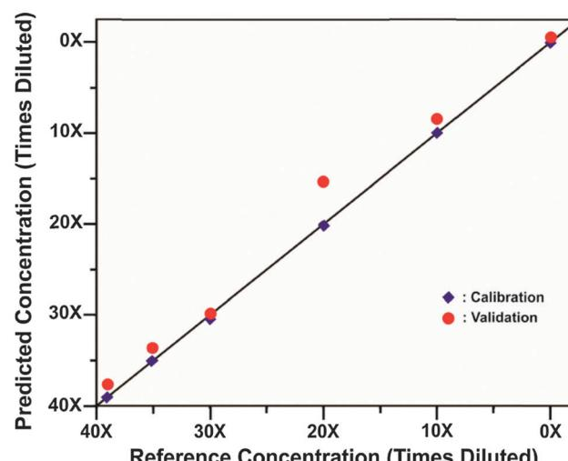
**Fig. 5** Calibration and validation data sets of SESORS quantitative measurements of BPE functionalized SERS nanotags through bone.<sup>53</sup> (Reprinted with permission from B. Sharma, K. Ma, M. R. Glucksberg, R. P. Van Duyne, *J. Am. Chem. Soc.*, 2013, **135**, 17290 Copyright (2013) American Chemical Society.)
