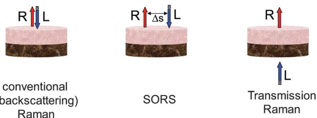
**Fig. 1** Schematic diagrams of basic Raman spectroscopy modalities: conventional backscattering Raman, SORS and Raman transmission geometries. Legend: R – Raman light, L – laser beam,  $\Delta s$  – spatial offset.
