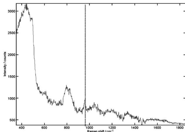
**Fig. 2** The recovered signal achieved for 0.125% (relative volume) of HAP buried within 20 mm of porcine tissue. The  $962\text{ cm}^{-1}$  peak is still clearly recognizable. Acquisition times were 5 s with 10 accumulations. Vertical line, HAP peak.<sup>34</sup> (Reprinted with permission from N. Stone and P. Matousek, *Cancer Res.*, 2008, **68**, 4424 with permission of the American Association for Cancer Research, Inc.)
