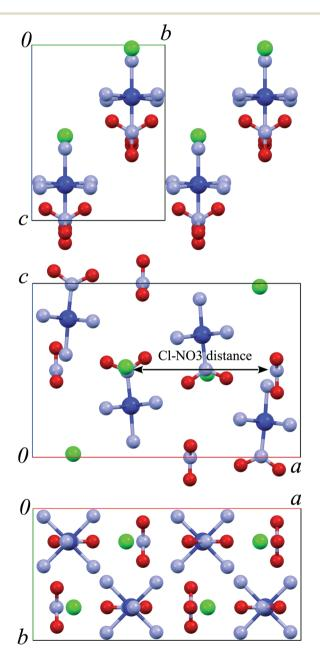
Fig. 1 The fragments of the crystal structure of  $[Co(NH_3)_5NO_2]Cl(NO_3)$  in different orientations. Chlorine anions are green, Co atoms dark blue, N atoms light blue, and oxygen atoms red. The complex hydrogen bond network (Fig. S3 and Table S2 in the ESI†) is not shown for clarity.
