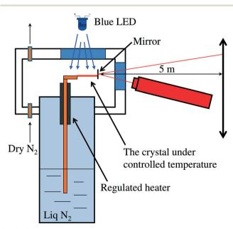
Fig. 2 Experimental set-up
