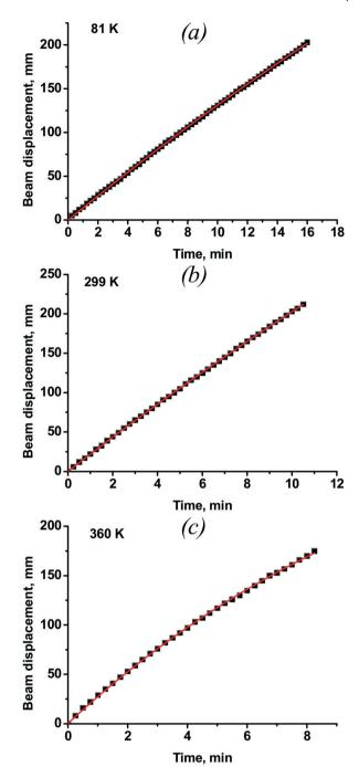
Fig. 5 The displacement of the laser beam during the bending of crystal #3 at variable temperatures: a) 81 K, b) 299 K, c) 360 K (data for other temperatures are available as ESI,† Fig. S1).
