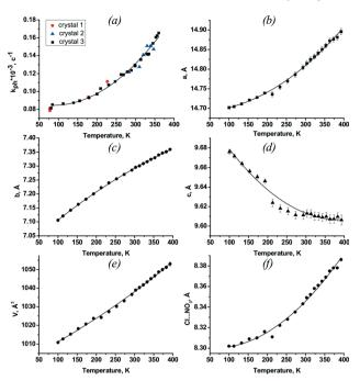
Fig. 6 The temperature dependences of: a) the rate constant of photoisomerisation  $k_{\rm ph}$ ; b–e) unit cell parameters a, b, c and volume V; f) the distance between the anions Cl and NO<sub>3</sub>, surrounding a nitroligand NO<sub>2</sub> (see Fig. 1).
