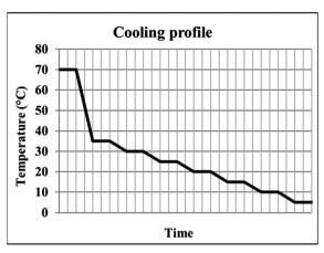
Fig. 2 The stepped cooling profile employed, showing the six regions of dwelling employed to ensure steady state is reached.
