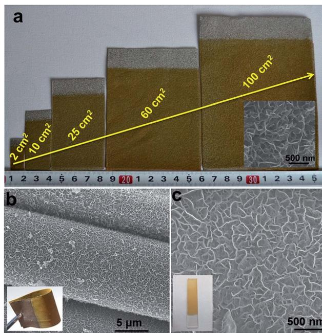
Fig. 5 (a) Photographs of NiFe-LDH nanoplatelet arrays synthesized on foam nickel substrates at various scales (inset: the SEM image of the NiFe-LDH sample on the  $100 \text{ cm}^2$  substrate); synthesis time for all the samples is 300 s at room temperature. SEM images for the NiFe-LDH nanoplatelet arrays on (b) a conducting cloth and (c) FTO substrate (inset: their corresponding photographs).
