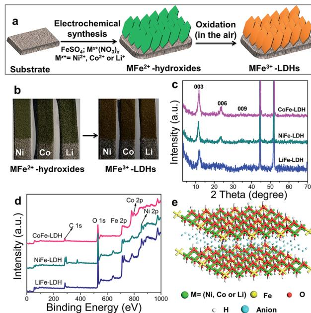
Fig. 1 (a) Scheme of the synthetic route to the MFe-LDH ( $M = \text{Co}, \text{Ni}$  and  $\text{Li}$ ) nanoarrays; (b) photograph of the MFe-LDH nanoarrays growing on the Ni foam before and after self-oxidation in the air; (c) XRD patterns and (d) XPS spectra of the MFe-LDH ( $M = \text{Ni}, \text{Co}$  and  $\text{Li}$ ) nanoplatelet arrays; (e) structure model of MFe-LDH.
