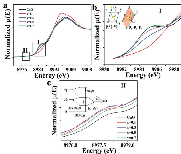
Fig. 3 (a) Normalized Cu–K edge XANES spectra for  $\text{Cu}_x\text{Ir}_{1-x}\text{O}_\delta$  compositions. (b) Shows the shakedown transition and the inset is a diagram of the Cu-4p orbital energy in two different symmetries. (c) Shows the amplified pre-edge region and the inset diagram shows the energy level of possible transitions. (b) and (c) correspond to the selected areas, I and II, in (a).
