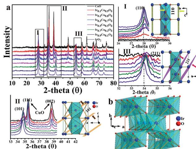
Fig. 2 (a) XRD patterns of the  $\text{Cu}_x\text{Ir}_{1-x}\text{O}_\delta$  compositions with different amounts of Cu doping. (I)–(III) correspond to the (a) selected areas. (b) Polyhedron picture of one  $\text{IrO}_2$  cell.
