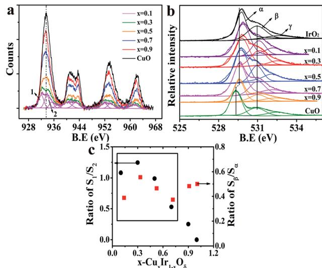
Fig. 4 (a) XPS spectra of Cu-2p in the  $\text{Cu}_x\text{Ir}_{1-x}\text{O}_8$  compositions with  $x = 0.1$  de-convoluted; other compositions' de-convoluted spectra are shown in the ESI. (b) XPS spectra of O-1s in the  $\text{Cu}_x\text{Ir}_{1-x}\text{O}_8$  compositions. (c) Pattern of the ratio of  $S_1/S_2$  and  $S_\beta/S_\alpha$  versus the doped amount  $x$ .
