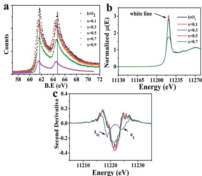
Fig. 5 (a) XPS spectra of Ir-4f in  $\text{Cu}_x\text{Ir}_{1-x}\text{O}_8$  compositions. The solid vertical lines correspond to the Ir-4f<sub>7/2</sub> and 4f<sub>5/2</sub> peak positions of  $\text{IrO}_2$ . (b) Normalized Ir-L<sub>III</sub> edge XANES spectra for  $\text{Cu}_x\text{Ir}_{1-x}\text{O}_8$  compositions. (c) Second derivatives of Ir-L<sub>III</sub> edge XANES spectra for  $\text{Cu}_x\text{Ir}_{1-x}\text{O}_8$  compositions.
