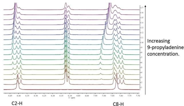
Fig. 3  $^1\text{H}$  NMR spectrum illustrating shifts in the C8-H and C2-H proton signals during titration of mono-TP with 9-propyladenine. Spectrum 1 corresponds to pure 9-propyladenine and spectra 2–17 are recorded with constant mono-TP concentration and increasing 9-propyladenine concentration.
