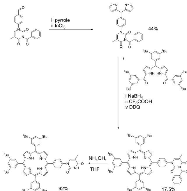
Scheme 2 Synthetic route used for the preparation of mono-TP.
