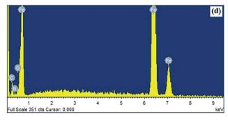
Fig. 9 (a–d) EDX images of mild steel: (a) in absence of AACs and in the presence of 40 mg  $\rm L^{-1}$  of (b) AAC-1, (c) AAC-2, and (d) AAC-3.
