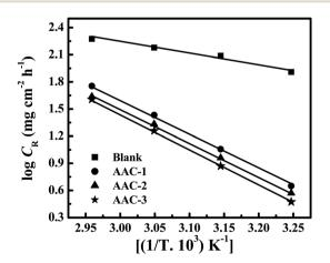
Fig. 3  $\,$  Arrhenius plots for the corrosion rate of mild steel  $\it versus$  the temperature in 1 M HCl.
