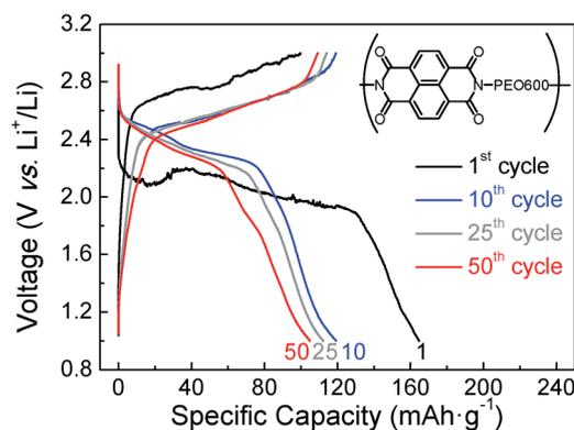
Fig. 9 Voltage profile for naphthalene polyimide-*b*-PEO600 at different cycle numbers at 1Li<sup>+</sup>/5 h rate.
