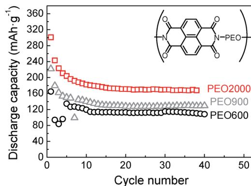
Fig. 10 Discharge capacities versus cycle number for naphthalene polyimide-*b*-PEO600 (○), naphthalene polyimide-*b*-PEO900 (△) and naphthalene polyimide-*b*-PEO2000 (□) at 1Li<sup>+</sup>/5 h rate.
