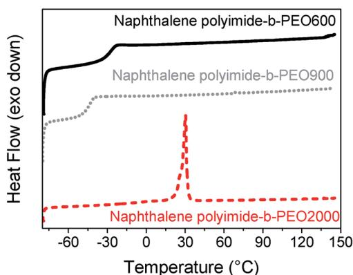
Fig. 3 DSC curves for naphthalene polyimides-*b*-PEO600 (black solid line), naphthalene polyimide-*b*-PEO900 (grey dot line) and naphthalene polyimide-*b*-PEO2000 (red dashed line) at 10 °C min<sup>-1</sup>.
