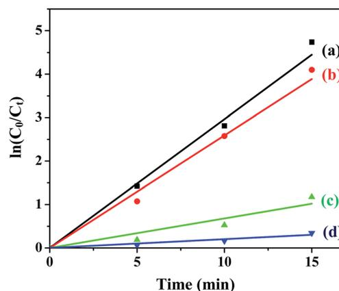
Fig. 7 Photodegradation kinetics of MB in the presence of (a)  $\text{CuFe}_2\text{O}_4$ , (b)  $\text{ZnFe}_2\text{O}_4$ , (c)  $\text{NiFe}_2\text{O}_4$  and (d)  $\text{CoFe}_2\text{O}_4$  under optimum conditions.
