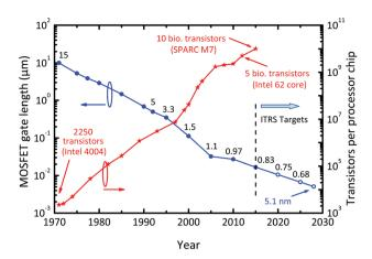
Fig. 2 Evolution of the MOSFET gate length and the number of transistors integrated on a single microprocessor chip. The numbers above the gate length curve indicate the processor supply voltage  $V_{\rm DD}$ . Note the continuous decrease of  $V_{\rm DD}$  in the past and the required continuation of this trend in the future. The ITRS targets refer to MOSFETs for high-performance logic as specified in the 2013 ITRS edition.<sup>7</sup>
