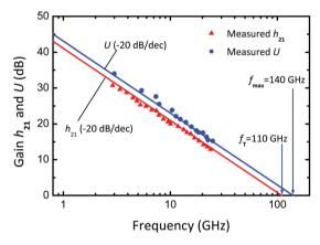
Fig. 6 Small-signal current gain  $h_{21}$  and unilateral power gain U of a RF FET as a function of frequency, after ref. 43 and 44. The characteristic frequencies  $f_T$  and  $f_{max}$  are obtained by extrapolating the measured  $h_{21}$ and U with the characteristic slope of -20 dB per dec.
