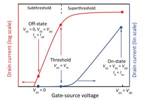
Fig. 5 Transfer characteristics of an n-channel FET showing the drain current  $I_D$  as a function of the gate-source voltage  $V_{GS}$  together with the on and off operating points for CMOS logic. Note that the scale of the left current axis is logarithmic and that of the right current axis is linear.
