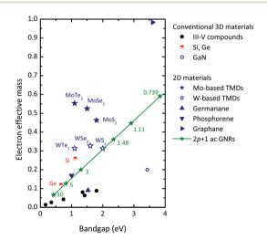
Fig. 12 Electron effective mass of 2D and conventional 3D semiconductors vs. bandgap. III-V compounds (black solid circles), from left to right InSb, InAs, In<sub>0.53</sub>Ga<sub>0.47</sub>As, InP, GaAs, Al<sub>0.3</sub>Ga<sub>0.7</sub>As. Data for TMDs and graphane from ref. 45, for germanane from ref. 53, for GNRs from ref. 135, and for phosphorene from ref. 136 and 137. The numbers at the GNR data points indicate the ribbon width according to the width-gap relationship from ref. 87.
