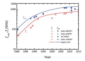
Fig. 3 Evolution of the cutoff frequency  $f_T$  and maximum frequency of oscillation  $f_{\text{max}}$  of RF FETs. Shown are the record  $f_{\text{T}}$  and  $f_{\text{max}}$  values reported at a certain time. MESFET: metal-semiconductor FET; HEMT: high electron mobility transistor; pHEMT: pseudomorphic HEMT; mHEMT: metamorphic HEMT. Data are taken from ref. 20-39.
