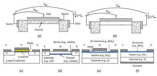
Fig. 4 Basic FET structures. Generic structure of a FET (a) in the on-state and (b) in the off-state. (c) Conventional Si n-channel MOSFET. (d) HEMT. (e) 2D MOSFET. (f) Back-gate 2D MOSFET frequently used for proof-of-concept purposes. Note that HEMTs and 2D MOSFETs do not possess pn junctions as present in conventional Si MOSFETs shown in (c) but rather resemble the junctionless MOSFET which is intensively investigated at present.42
