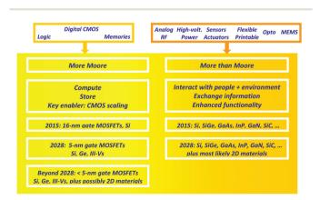
Fig. 1 The More Moore and More Than Moore domains of semiconductor electronics, together with important trends and the semiconductors used in these domains. Note that the year 2028 indicates the end of the time horizon of the 2013 ITRS edition.
