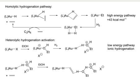
Scheme 6 Computational modelling of Au(i) mediated hydrogenation steps (L = IPr)
