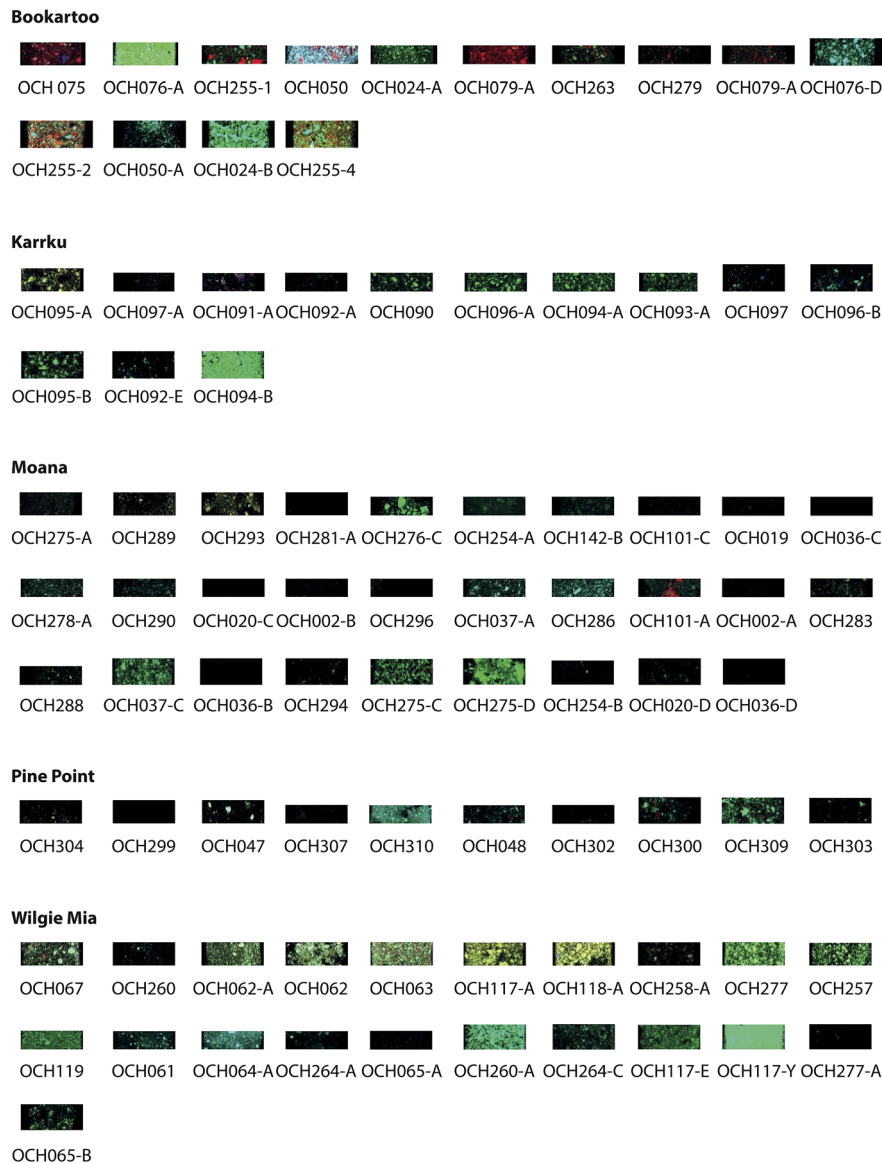
Fig. 6 Microelemental map of Ca, Fe and V for samples from the sites analysed in this study. Red indicates Ca, green indicates Fe and blue indicates V. Images are false coloured to demonstrate relative concentration intensities, with black the lowest and the indicated colour the highest. Sites are highlighted in each image. (a) Bookartoo (b) Karrku (c) Moana (d) Pine Point (e) Wilgie Mia.
