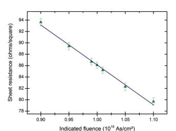
**Fig. 4** Sensitivity of sheet resistance to fluence. The indicated implanted fluence is used here with all the implants ( $1\times10^{15}$  As cm $^{-2}$ ,  $\pm1\%$ ,  $\pm5\%$ ,  $\pm10\%$ ) done at the same time. All 7 wafers are annealed at the same time: 3 minutes RTA at 950 °C. The vertical error bars are given as the standard deviation of 197 measurements performed on each wafer. Linear regression is also shown on the figure (blue line).
