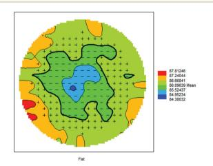
Fig. 3 Typical sheet resistance uniformity by 4pp for As fluence of 1 TFU. For this wafer the average sheet resistance non-uniformity (standard deviation of 197 measurements with 5 mm spacing) is 0.8. None of the QA wafers measured in this work had a non-uniformity >0.84%. Average sheet resistance is  $86.1~\Omega/\Box$  (equivalent to  $1.00\times10^{15}$  As cm<sup>-2</sup> from the calibration curve in Fig. 4).
