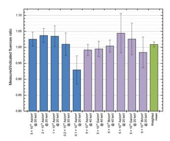
Fig. 9 RBS of various implants into 11 samples. 11 separate samples were implanted on the Danfysik tool under various conditions (see labels), and directly verified by RBS using 2.0 MeV <sup>7</sup>Li<sup>2+</sup> (in purple) or 1.5 MeV <sup>4</sup>He<sup>+</sup> (in blue) incident beam. The error bars show the combined standard measurement uncertainty in each fluence measurement. The standard error of the weighted mean (in green) is 0.83%. See Table 3 for data.
