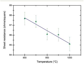
Fig. 5 Sensitivity of sheet resistance to anneal temperature. 3 minutes RTA at various temperatures. The same indicated implanted fluence of  $10^{15}$  As cm $^{-2}$  is used here with all the 5 implants done at the same time. The vertical error bars are given as the standard deviation of 197 measurements performed on each wafer. Linear regression is also shown on the figure (blue line).
