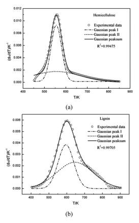
**Fig. 3** DTG curves of hemicellulose and lignin based on multi-peaks method.
