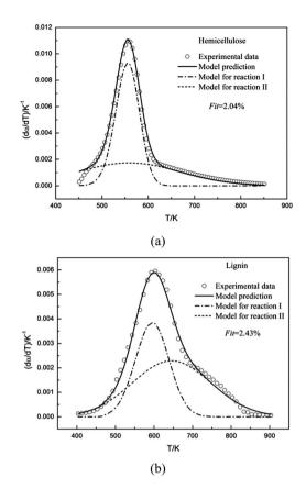
Fig. 4 Experimental and calculated DTG curves of hemicellulose and liquin.
