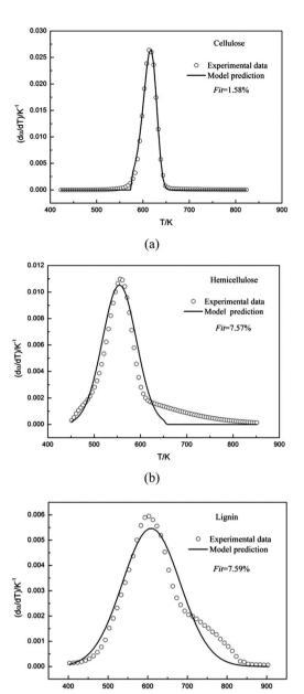
Fig. 2 Experimental and calculated DTG curves of cellulose, hemicellulose and lignin using the single Gaussian-DAEM-reaction model.
