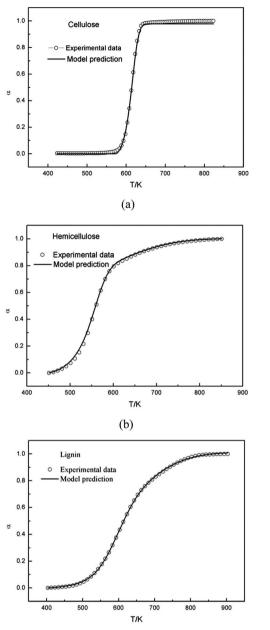
Fig. 5 Experimental and calculated  $\alpha(T)$  curves of cellulose, hemicellulose and lignin by integrating the calculated DTG curve.
