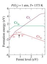
**Fig. 3** Calculated formation energy as a function of  $\varepsilon_F$  for Cr-related defects under a realistic growth condition ( $\mu_O = -1.57$  eV). The arrow indicates the estimated pinned  $\varepsilon_F$ . The slope of each line indicates the charge state. The transition levels between different charge states are denoted as kinks in each plot.
