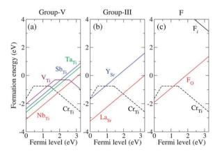
**Fig. 4** Calculated formation energies as a function of  $\varepsilon_F$  for (a) group-V codopants (Nb, Ta, Sb, and V), (b) group-III codopants (La and Y), and (c) F, as well as  $Cr_{Ti}$  in each case. All formation energies were calculated for  $\mu_O=-1.57$  eV.
