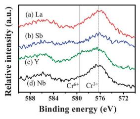
Fig. 7 X-ray photoelectron spectra of Cr 2p of (a) La–Cr, (b) Sb–Cr, (c) Y–Cr, and (d) Nb–Cr codoped SrTiO $_3$ . The peaks assigned to  $Cr^{3+}$  and  $Cr^{6+}$  are indicated by dashed and dotted lines, respectively.
