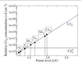
Fig. 5 Calculated relative concentration of Cr<sub>Ti</sub> defects, derived from hypothetical formation energies, as a function of Fermi level ( $\varepsilon_F$ ). The pinned  $\varepsilon_F$  results from the charge-neutrality condition for codoped (circles) and non-codoped (square) Cr-doped STO.
