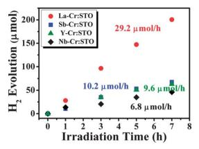
Fig. 6 Photocatalytic H<sub>2</sub> evolution from water splitting of Cr and D codoped  $SrTiO_3$  under visible light irradiation, where D = La, Sb, Y, and Nb. All codoped samples were prepared using 5 mol% of Cr and 5 mol% of D.
