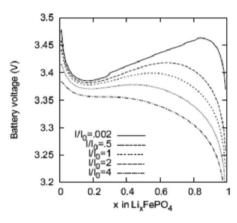
Fig. 14 Top) calculated phase separation in a particle which has been allowed to relax from a homogeneous state at zero current with stress-free boundaries. White regions are lithium-rich. Down) Calculated LIB voltage at different applied currents. Reprinted with permission from ref. 169. Copyright 2011, The Electrochemical Society.
