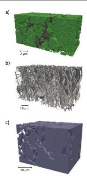
**Fig. 29** 3D reconstructions obtained by FIB tomography of (a) a LiFePO $_4$  composite positive electrode, (b) a glass fiber separator and (c) a graphite negative electrode. Reprinted with permission from ref. 231. Copyright 2012, The Electrochemical Society.
