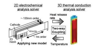
Fig. 35 Schematics of the electrochemical-thermal on-the-fly coupled simulation method of LIBs. Reproduced with permission from ref. 260. Copyright 2012, The Electrochemical Society.
