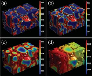
**Fig. 30** Li concentration (mol cm $^{-3}$ ) evolution during the discharge of a Li<sub>x</sub>CoO<sub>2</sub> microstructure at a constant voltage loading. Through electrochemical reaction, Li ions are injected into cathode particles: (a)–(d) corresponding to time of 4.04, 20.1, 133.3 and 1226.5 s (assuming the value of the diffusion coefficient of  $10^{-10}$  cm $^2$  s $^{-1}$ ). Reprinted with permission from ref. 234. Copyright 2012, The Electrochemical Society.
