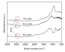
**Fig. 7** FTIR absorption spectra of the nanoparticles after being fluidized in the presence of ISP vapour. The peaks at 2976 cm<sup>-1</sup> correspond to the stretching vibration of CH<sub>3</sub> groups in the isopropanol molecule.<sup>26</sup>
