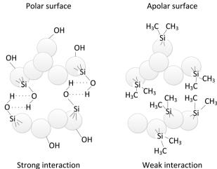
Fig. 1 Sketch of the particle-particle interaction for polar and apolar SiO<sub>2</sub> nanoparticles.
