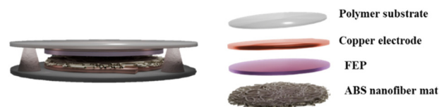
Fig. 2 Schematic representation of the ABS-based TENG.
