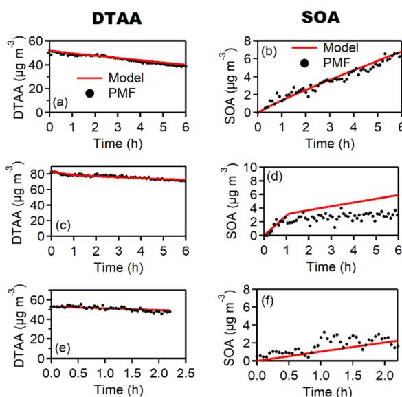
Fig. 10 Comparison of model predictions (red line) and experimental measurements (black dots) (in  $\mu\text{g m}^{-3}$ ) for three representative oxidation experiments: (a and b) Experiment 6 (low- $\text{NO}_x$ , FORTH-ASC), (c and d) Experiment 7 (high- $\text{NO}_x$ , FORTH-ASC), and (e and f) Experiment 9 (high- $\text{NO}_x$ , CMU-ASC). Panels show pure DTAA and secondary organic aerosol (SOA) formation over time.
