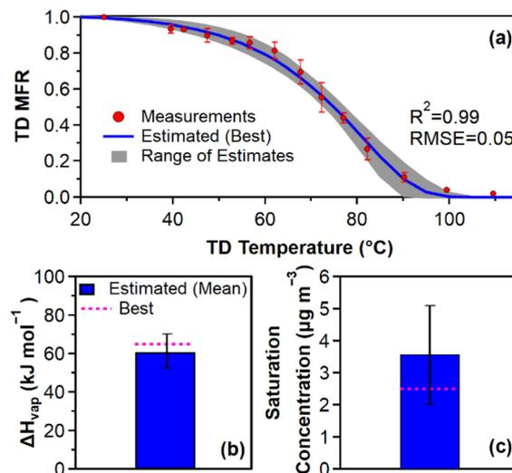
Fig. 4 (a) MFR after the TD for AMS measurements (red dots), the model average prediction (blue line), and the range of model estimates (grey area); (b) the mean estimated  $\Delta H_{\text{vap}}$  (blue bar) and its best estimate (dashed pink line); and (c) the mean estimated  $C^*$  (blue bar) and its best estimate (dashed pink line). The measurements have been corrected for size- and temperature-dependent particle losses. The error bars correspond to one standard deviation.
