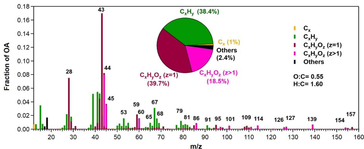
Fig. 2 HR average AMS spectrum of pure diaterpenylic acid acetate (DTAA) aerosol. The most important characteristic  $m/z$  ratios were 53, 59, 60, 65, 67, 68, 69, 71, 77, 79, 80, 81, 82, 85, 86, 91, 95, 101, 109, 114, 126, 127, 139, 154 and 157.
