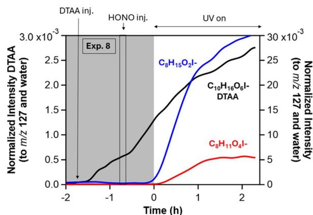
Fig. 9 CIMS time-series of DTAA (left y-axis) and products (right y-axis) for Exp. 8.
