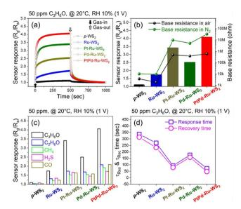
Fig. 20 (a) Sensing plots of various gas sensors to  $C_3H_6O$ , (b) corresponding response, and baseline resistance in air and  $N_2$ ; (c) selectivity curves, and (d) response and recovery times. Reproduced with permission from Elsevier, ref. 92.
