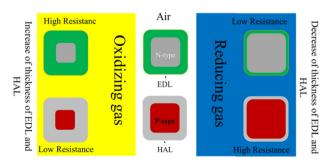
Fig. 4 General gas sensing mechanism of n- and p-type resistive gas sensors in the presence of oxidizing and reducing gases.
