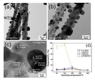
Fig. 9 (a) and (b) TEM and (c) HRTEM images of AuPd–ZnO NWs and (d) response of gas sensors to 1 ppm  $NO_2$  versus temperature. Reproduced with permission from Elsevier, ref. 60.
