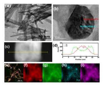
Fig. 12 (a) TEM image of  $W_{18}O_{49}$  NWs, (b) HRTEM image of  $W_{18}O_{49}$  NWs/BNPs-2 and (c) and (d) EDS elemental line and (e)–(i) surface scans of  $W_{18}O_{49}$  NWs/BNPs-2. Reproduced with permission from Elsevier, ref. 72.
