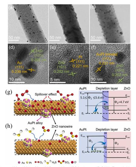
Fig. 16 TEM and HRTEM images of (a) and (d) Au-, (b) and (e) Pt-, and (c) and (f) PtAu-decorated ZnO NWs. The underlying H<sub>2</sub>S sensing mechanism of the PtAu-decorated ZnO NWs in (g) air and (h) H<sub>2</sub>S gas. Reproduced with permission from Elsevier, ref. 76.
