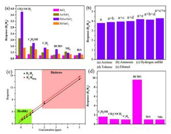
Fig. 11 Sensing tests of the AuPd/SnO<sub>2</sub> sensor: (a) selectivity graph; (b) discrimination test of the response to the mixed gas (1 ppm C<sub>3</sub>H<sub>6</sub>O and 1 ppm other interference gases); (c) response to different concentrations of C<sub>3</sub>H<sub>6</sub>O in a 94% RH environment at 250 °C; and (d) AuPd/SnO<sub>2</sub> sensor selectivity at 110 °C. Reproduced with permission from Elsevier, ref. 65.
