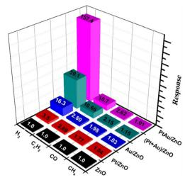
Fig. 15 Selectivity of various gas sensors to 250 ppm gases at 130 °C. Reproduced with permission from Elsevier, ref. 75.
