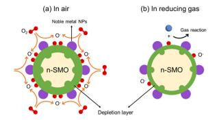
Fig. 5 Catalytic effect of noble metals for enhanced gas response of resistive gas sensors
