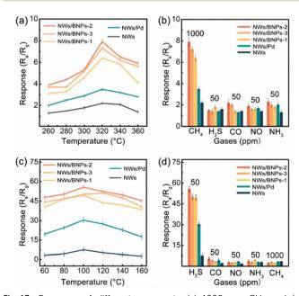
Fig. 13 Response of different sensors to (a) 1000 ppm CH $_4$  and (c) 50 ppm H $_2$ S *versus* temperature; selectivity of W $_{18}$ O $_{49}$  NWs/BNPs-2 at (b) 320 °C and (d) 100 °C. Reproduced with permission from Elsevier, ref. 72.
