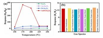
Fig. 10 (a) Gas sensing response of various gas sensors to 100 ppm  $C_3H_9N$ ; (b) selectivity of the AuPd-In<sub>2</sub>O<sub>3</sub> sensor to 10 ppm gas and 10 ppm  $C_3H_9N$ . Reproduced with permission from Elsevier, ref. 61.
