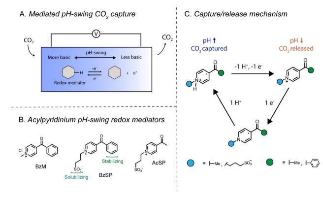
Fig. 1 (A) General scheme for redox-mediated pH-swing carbon capture in one compartment. (B) Acylpyridinium redox mediators used in this work. (C) Mechanism of  $CO_2$  capture with pyridinium mediators.
