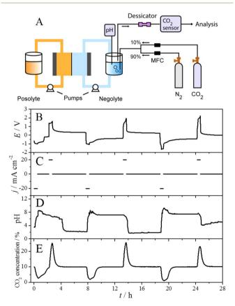
Fig. 4 (A) Schematic diagram of the flow cell system used in the pHswing CO<sub>2</sub> capture/release test. (B-E) Variation of the cell potential (B), current density of WE (C), pH of negolyte (D) and CO<sub>2</sub> concentration in the gas outlet (E) as a function of time during the CO<sub>2</sub> capture/release test
