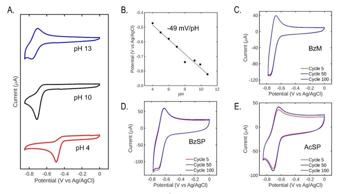
Fig. 2 Cyclic voltammetry of 5 mM pyridinium mediators at 100 mV s $^{-1}$  under argon. (A) Cyclic voltammograms of BzM in various buffers with 1 M KNO<sub>3</sub>. (B) Pourbaix diagram of BzM. (C-E) Long-term cyclic voltammograms in unbuffered 1 M KNO<sub>3</sub> of BzM, BzSP, and AcSP.
