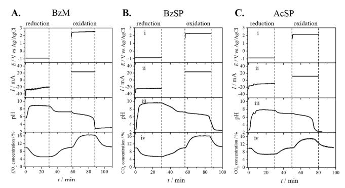
Fig. 3 H-cell  $CO_2$  capture/release tests. (A–C)  $CO_2$  capture/release results in the H-cell, (A) BzM, (B) BzSP, (C) AcSP. Fumasep AEM was used for BzM, and Nafion CEM was employed in the test of BzSP and AcSP. The pyridinium mediators were reduced using a constant potential and were reoxidized using a constant current. (i) Applied potential on the Pt WE, (ii) current of the Pt WE, (iii) pH of electrolyte in the WE compartment and (iv)  $CO_2$  concentration in the gas outlet.
