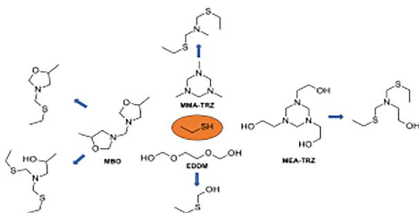
**Characterization of products from the chemical removal of thiol in hydrocarbon streams using DART-MS and NMR spectroscopy**Rolando Perez Pineiro,\* Jody Hoshowski,
