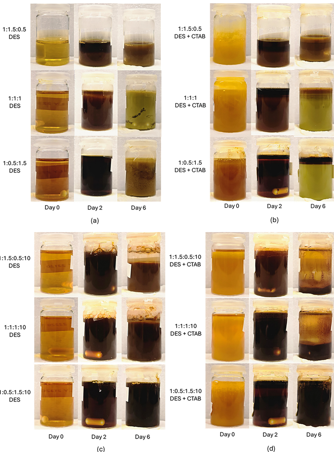
Fig. 1 Pictures of \text{Fe}(\text{NO}_3)_3 dissolved in unhydrated and hydrated DES kept at 70^\circ\text{C} . (a) \text{Fe}(\text{NO}_3)_3 in unhydrated DES w/o CTAB, (b) \text{Fe}(\text{NO}_3)_3 in unhydrated DES w/CTAB, (c) \text{Fe}(\text{NO}_3)_3 in hydrated DES w/o CTAB, and (d) \text{Fe}(\text{NO}_3)_3 in hydrated DES w/CTAB. The pictures are taken at day 0, day 2 and day 6 after dissolving the salt. The nanoparticles were separated by injecting this solution into DI water, after 7 days stored at 70^\circ\text{C} , after dissolving the salt.
