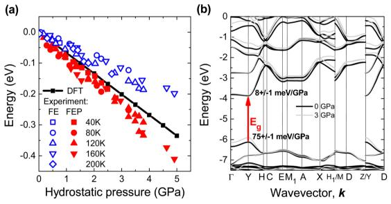
Fig. 6 (a) Relative changes in the position of the FE (blue points) and FEP (red points) peaks in EA<sub>2</sub>PbI<sub>4</sub> as a function of hydrostatic pressure and changes in the energy gap obtained from DFT calculations. (b) Electronic band structure of EA<sub>2</sub>PbI<sub>4</sub> without hydrostatic pressure (black lines) and under hydrostatic pressure (gray lines).
