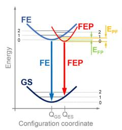
Fig. 2 Configuration diagram for free exciton and FE-polaron transition in EA<sub>2</sub>PbI<sub>4</sub>.
