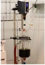
Chart 1 The 5 L stirred reactor used for the upscaled synthesis of lignin LPO
