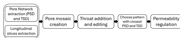
Fig. 1 Proposed steps for rock pattern design method.
