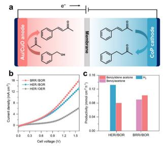
Fig. 6 (a) Schematic illustration of the coupling reaction system. (b) LSV curves of the HER//OER system, HER//BOR system and BRR//BOR system at a scan rate of 10 mV s<sup>-1</sup>. (c) Productivities of different products in the three electrocatalytic systems at a cell voltage of 1.5 V.
