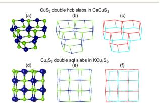
Fig. 3 (a-c) Double hcb and (d-e) double sql slabs in the structures of charge-balanced CaCuS<sub>2</sub> and charge-unbalanced KCu<sub>4</sub>S<sub>3</sub> phases, respectively.
