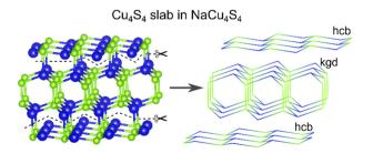
Fig. 4 Cu<sub>4</sub>S<sub>4</sub> slab in the NaCu<sub>4</sub>S<sub>4</sub> structure made from four hcb layers. Two central layers are connected in kagome dual net motif (kgd).
