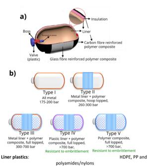
Composites: Glass/ carbon fibre composites with epoxy, polyesters, phenolics, polyamides and polyphenylene sulphide.
