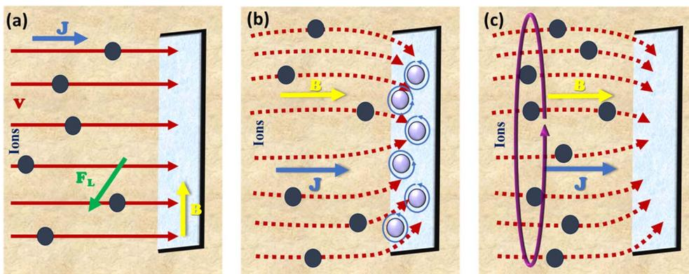
Fig. 6 Illustration of the magnetic field effects in an electrocatalytic system, showing the relationship between current density,  $J$ , magnetic field,  $B$  and Lorentz force,  $F_L$ : (a)  $J$  is normal to the electrode surface and  $B$  is parallel, (b) both  $J$  and  $B$  are normal to the surface with MHD flow appearing at the corners and (c) micro MHD action developed in the system.
