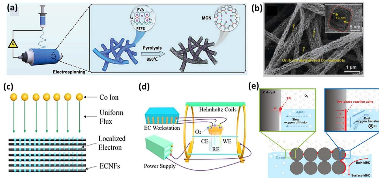
Fig. 23 (a) Schematic of using sol-gel electrospinning and pyrolysis. (b) Surface image of magnetic nanocages with the inset showing a single Co nanodot (reprinted with permission,<sup>217</sup> copyright 2020, Wiley). (c) Schematic of the uniform deposition of  $\text{Co}^{2+}$  and (d) schematic depiction of generating a magnetic field with Helmholtz coils and analysis of ORR (reprinted with permission,<sup>218</sup> copyright Wiley).
