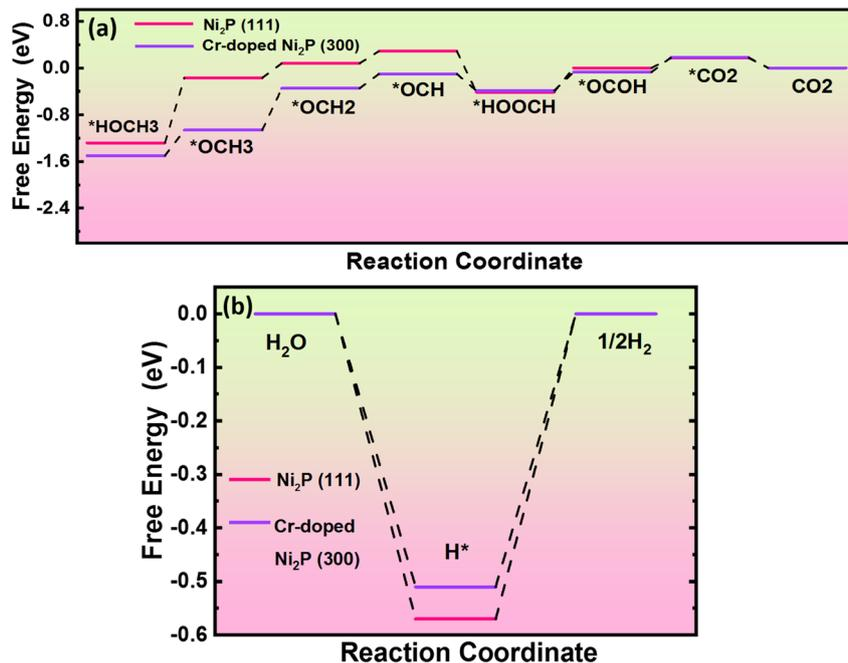
Fig. 4 Free energy diagrams: (a) Gibbs free energy diagrams of undoped  $\text{Ni}_2\text{P}$  (111) and Cr-doped  $\text{Ni}_2\text{P}$  (300) for the MOR. (b) Hydrogen adsorption free energy diagrams of undoped  $\text{Ni}_2\text{P}$  (111) and Cr-doped  $\text{Ni}_2\text{P}$  (300) for the HER.
