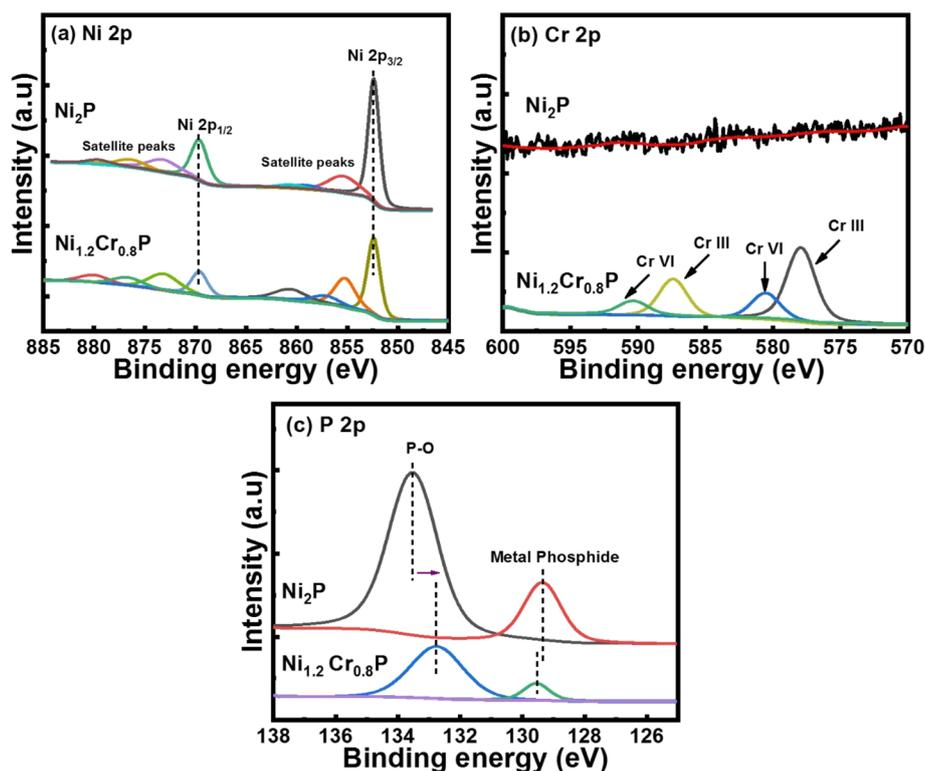
Fig. 2 High-resolution core-level XPS spectra of (a) Ni 2p, (b) Cr 2p and (c) P 2p in Ni<sub>1.2</sub>Cr<sub>0.8</sub>P NRs.
