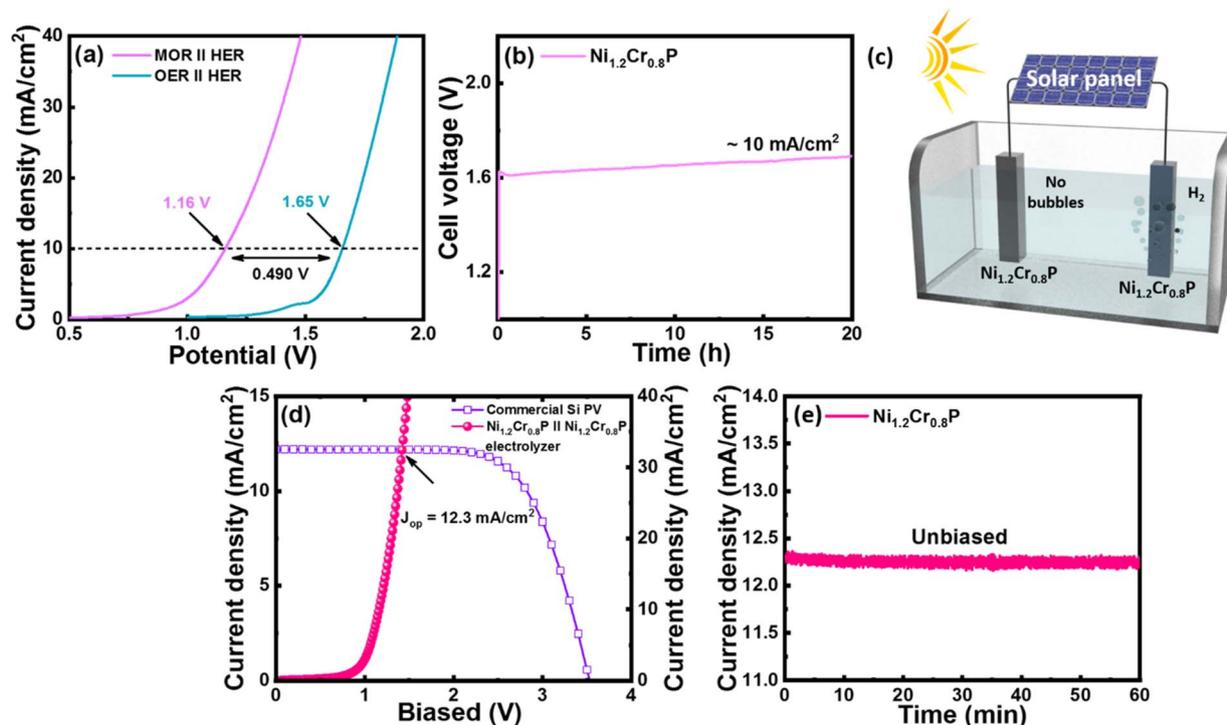
Fig. 5 (a) Comparison of polarization curves for OMeS (MOR||HER) in 1.0 M KOH/3 M MeOH and OWS (OER||HER) in 1 M KOH using  $\text{Ni}_{1.2}\text{Cr}_{0.8}\text{P}$  electrocatalysts as both an anode and a cathode. (b) Long-term durability test of OMeS for 20 h. (c) Schematic representation of a solar-driven electrolysis cell. (d) Solar-to-hydrogen (STH) efficiency plot for the OMeS system (e) Unbiased water splitting photocurrent measured for 60 min in the OMeS system.
