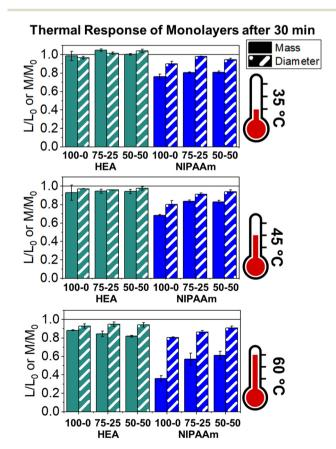
Fig. 3 Thermal response of pNIPAAm and pHEA monolayer hydrogels at 35, 45, and 60  $^{\circ}$ C. Ratio of hydrogel diameter and mass after 30 minutes in a water bath at 35, 45, and 60  $^{\circ}$ C relative to the initial length or mass.
