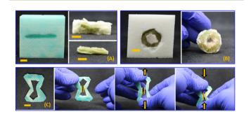
Fig. 4 Demonstration of cured composites of HEA in foam by HIFU curing: (A) a single post as cured and after extraction from the foam, (B) a ring as cured and after extraction from the foam, and (C) an auxetic design after extraction from the foam and under tension. Scale bars = 1 cm.
