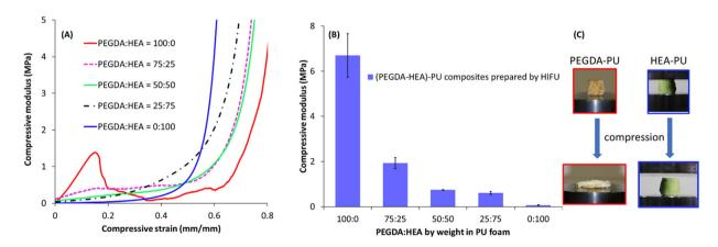
Fig. 10 (A) Uniaxial compression tests on composites made from foams with PEGDA, HEA, and mixtures of PEGDA and HEA, (B) compressive modulus data of the composites at different weight fractions of PEGDA and HEA (see Table S3†), (C) pictures showing PEGDA-foam and HEA-foam composites before and after compression.
