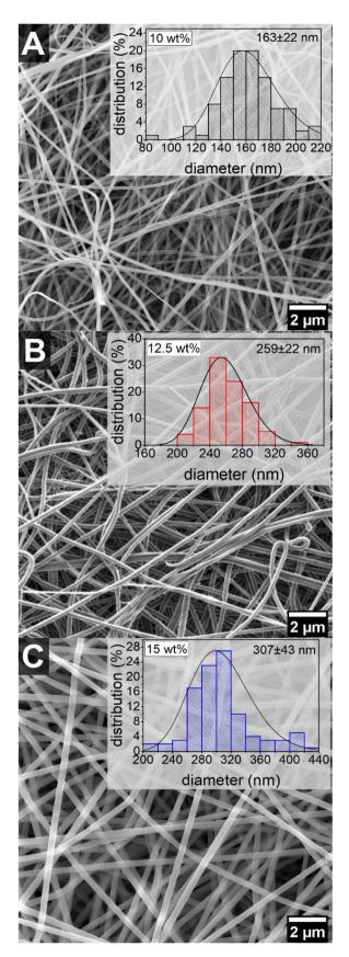
Fig. 1 SEM images and fiber diameter distributions of EFMs prepared from (A) 10 wt%, (B) 12.5 wt% and (C) 15 wt% solutions of PA 6.9 in formic acid/chloroform 1:1 v/v.
