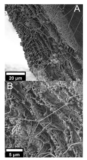
Fig. 4 SEM pictures of the cross section of the PA 6.9\_12.5 wt% membrane after filtration, (A) at 1000× magnification and (B) at 3500× magnification.
