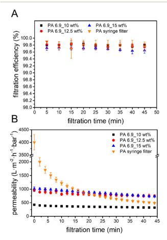
Fig. 3 (A) Filtration efficiency and (B) permeability over time for PS-MP removal using the bio-based EFMs and the PA syringe filter at 1 mL  $min^{-1}$ .
