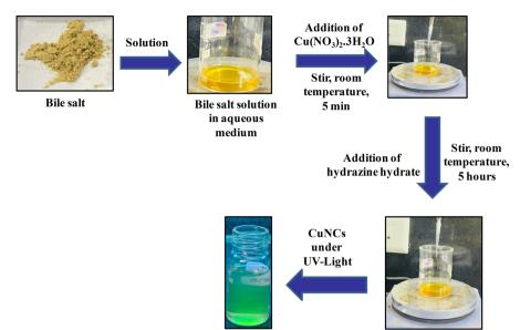
Scheme 1 Synthesis of CuNCs using bile salt templates.
