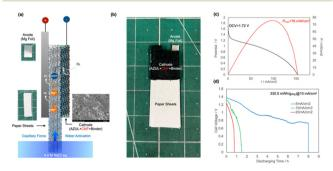
Fig. 3 Schematic of a completely disposable water-activated paper battery cell (a), a photograph of a disposable water activated paper battery (b), and its I-V/I-P polarization curves (c) and discharge polarization curves at different current densities (d), respectively. The inset in (a) shows an SEM image of the cathode containing CNFs.
