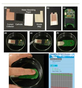
Fig. 4 Photographs of cell components (a), a single paper battery cell (b), SpO<sub>2</sub> sensor (c), SpO<sub>2</sub> sensor with the cell (d), injection of salt water to the cell (e), and the active  ${\rm SpO}_2$  sensor (other side compared with panels (d) and (e)) (f). Real-time monitoring of O2 saturation and pulse measured in a person (g).
