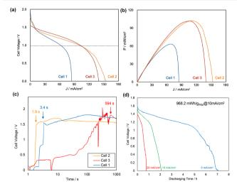
Fig. 2 I-V (a) and I-P (b) polarization curves of the cells (cell 1 (blue), cell 2 (yellow), and cell 3 (red)), time dependence of cell voltages of the cells after water activation (c), and discharge polarization curves of cell 2 at 5 (blue), 10 (green), and 20 mA cm $^{-2}$  (red) (d).
