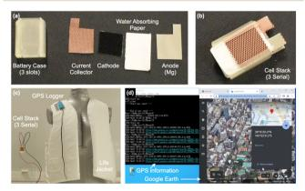
Fig. 5 Photographs of the cell components (a), the cell stack with three serial paper battery cells (b), and the arrangement of GPS loggers and the cell stack (c). A capture of the desktop showing the GPS information from the GPS logger activated by the cell stack with salt water and the detailed information obtained from Google Earth via GPS information (d).
